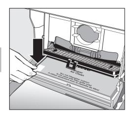
■ Insert a new "Air Clean" filter. It can be inserted with either side up.
