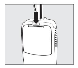
Remove the filter at the clean space (see arrow) and replace it with a new one.
