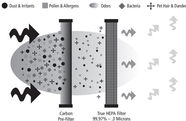
Above is an illustration of how the ***QuietFlo*<sup>®</sup>** True HEPA Air Purifier works. Dust and other irritants are pulled into the air purification system and cleaned through the HEPA Filter. Clean, purified air is released into the room.
