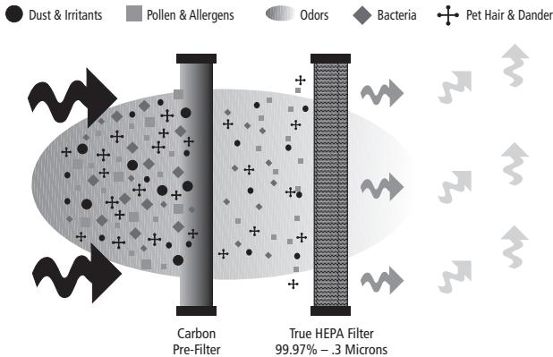
Above is an illustration of how the ***QuietFlo*®** True HEPA Air Purifier works. Dust and other irritants are pulled into the air purification system and cleaned through the HEPA Filter. Clean, purified air is released into the room.
