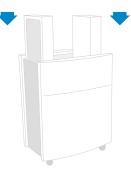
STEP 5: Place the third filter on top of the unit and ensure that the black side or the mark "out" is
